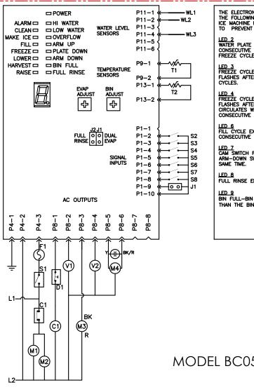
THE ELECTRONIC CONTROL WILL MONITOR FOR THE FOLLOWING CONDITIONS AND PREVENT THE ICE MACHINE FROM OPERATING AS REQUIRED TO PREVENT DAMAGE.
