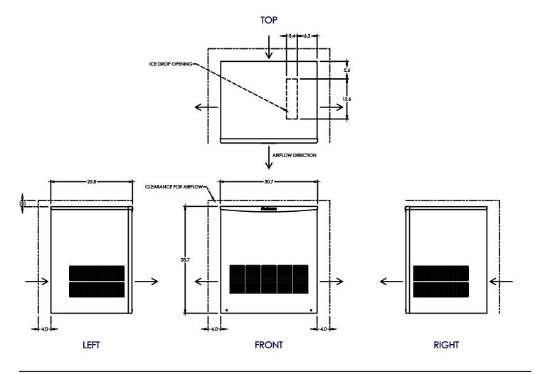
Note: Do NOT install on a bin where the ice drop opening is blocked.
